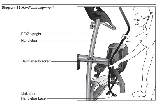
Note: Perform the following steps on one handlebar at a time.
